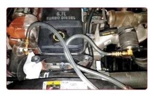
On 2015 and newer CAB Chassis trucks unbolt the crossover tube flanges and rotate the crossover tube down allowing access for bolted flange adapters #ZW21004 and ZW21005.
